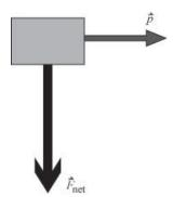
The diagram shows the momentum of an object and the net force acting on it at some instant in time. (You may assume the force is constant.)
